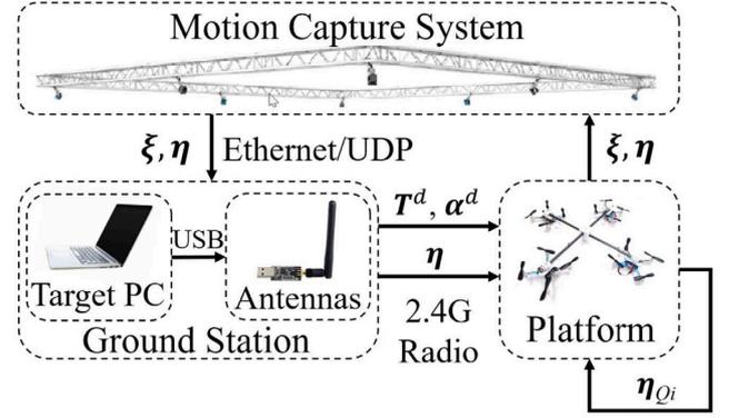
**Fig. 4.** Experiment setup. The motion capture system measures the position and attitude of the platform central frame, and send the data to the target PC through Ethernet, where the position and attitude controllers in addition to the input allocator run. The inner-loop reference signals are sent to each quadcopter through 2.4G radio. The inner-loop tracking controllers run onboard each quadcopter.
